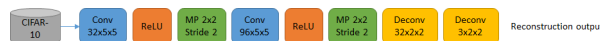
Figure 3: A CIFAR-10 autoencoder. A pair of these is used as a benchmark for the CIFAR-10 joint autoencoder.
