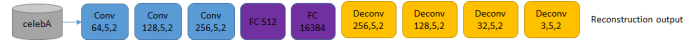
Figure 5: A celebA autoencoder. A pair of these is used as a benchmark for the celebA joint autoencoder.
