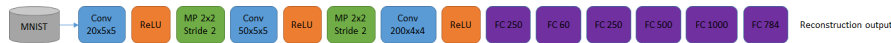
Figure 1: An MNIST autoencoder. A pair of these is used as a benchmark for the MNIST joint autoencoder.
